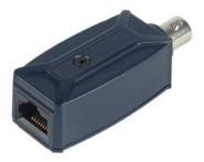
IP01 is a low cost and easy, speedy solution to allow you use existing coax cable to send IP camera signal. Used in pairs with your RG59 cable to exceed the IEEE 802.3 10BaseT specification. The working range could up to 200 meters at 10Mbps speed.
