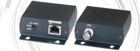
PTA-IP01P Extender is designed to send and extend IP/POE camera or any TCP/IP 10/100 BaseT devices over existing coax cable. The distance could up to 300 meters by RG6U 75 $\Omega$  Coaxial Cable. They are completely transparent to protocols, codes, and applications ensuring compatibility with any IP, POE camera and its management software. It is perfect solution to replace the analog camera to IP/POE camera using existing coax cable.
