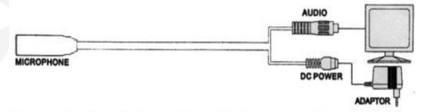
Remark: Since Hi sensitivity microphone, PTA-1103/R audio pick up box must be put at 5 meters away from monitor to avoid any audio reverberation.
